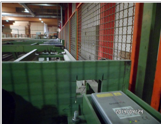
Pic 1: Dimetix Laser measures the wood face-on
